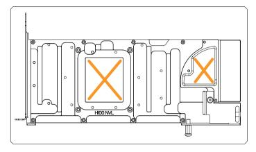
Apply the enclosed EK-TIM Ectotherm thermal grease (thermal compound) on the GPU heat spreader – IHS – as shown in the image. The layer of the thermal compound must be thin and even over the entire surface of the IHS.
