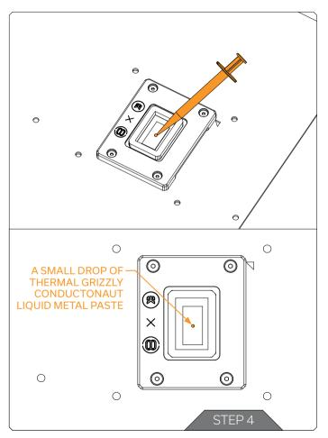
Apply a small drop of Thermal Grizzly Conductonaut liquid metal paste and spread it evenly over the DIE with cotton swabs that are included in the bag. Use the provided needle accessory that is included in the bag. Don't press the syringe too hard!
