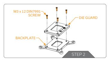
Separate the Die Guard from the Backplate by unscrewing four (4) M3 x 12 DIN7991 Screws. **Save the parts for later use.**
