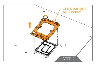
Remove the CPU mounting mechanism from the motherboard. The stock backplate must also be removed.
