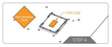
Before applying the Liquid Metal, clean the CPU DIE using a non-abrasive cloth or Q-Tip.
