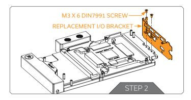
Position the replacement I/O Bracket on the water block. During this process, make sure you have aligned the holes. Secure it with the two (2) M3 x 6 DIN7991 Screws and Allen Key 2 mm.
