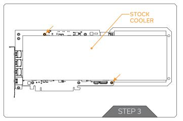
From the front side of the GPU, an additional two (2) screws must be removed (using Phillips head screwdriver). Detach the GPU Backplate.
