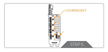
Lastly, unscrew five (5) Screws and detach the I/O Bracket (using Phillips head screwdriver).
