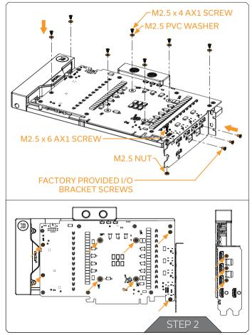
Use seven (7) M2.5 x 4 AX1 Screws and PVC washers to tighten the PCB on the water block. Tighten the screws evenly using the Phillipshead screwdriver. An additional one (1) M2.5 x 6 AX1 Screw must be secured with an M2.5 Nut.
