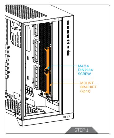
EK provides a Kinetic<sup>3</sup> Side Mount Bracket along with M4 nuts, washers and screws to allow the installation of the reservoir onto fans, radiators or PC cases. The bracket can be positioned across any pair of mounting holes in various orientations.
