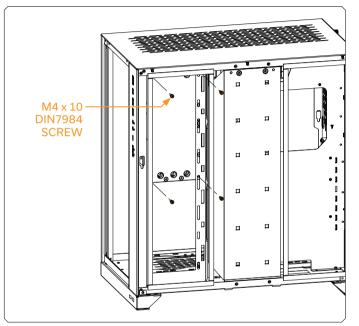
Using the included M4 screws you can mount the reservoir directly to your chassis or any other standard fan mounting location.
