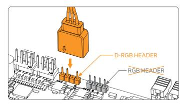
Plug the 3-pin connector from the water block's D-RGB LED light in the D-RGB HEADER on the motherboard. The LED will work if the pin layout on the header is as follows: +5V, Digital.
