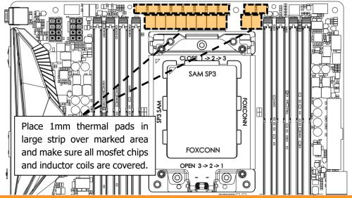
Prior to fastening the screws please make sure the mounting holes on the motherboard's circuit board are aligned with the water block. Secure top 4 (four) nickel screws with enclosed 2,5mm Allen key. Tighten screws diagonally and evenly till the end of the thread. Do not use excessive force when tightening the screws!
