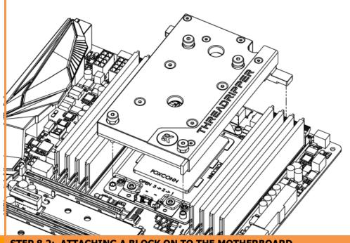
Prior to fastening the screws please make sure the mounting holes on the motherboard's circuit board are aligned with the water block. Use 2 (two) M2,5x5 AX1 screws with M2.5 PVC washers. Tighten the screws evenly. Do not use excessive force when tightening the screws!
