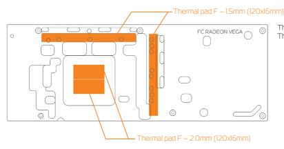
Thermal pad F – 2.0mm (120x16mm) – (EAN: 3830046996756) Thermal pad F – 1.5mm (120x16mm) – (EAN: 3830046996749)
